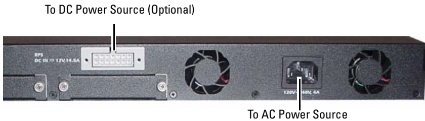
Figure 1-15. AC and DC Power Connection to Switch
